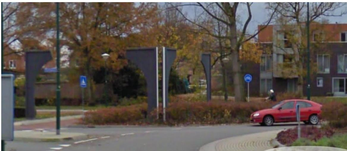
**Figure 3: Roundabout with obstructed view for the vehicle.**
